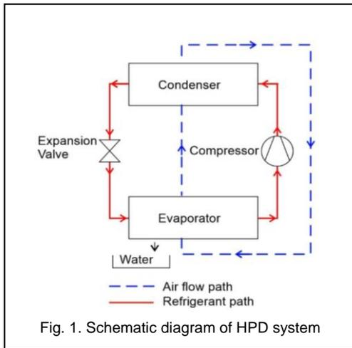
Fig. 1. Schematic diagram of HPD system
