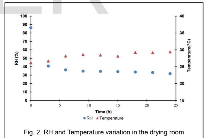
Fig. 2. RH and Temperature variation in the drying room
